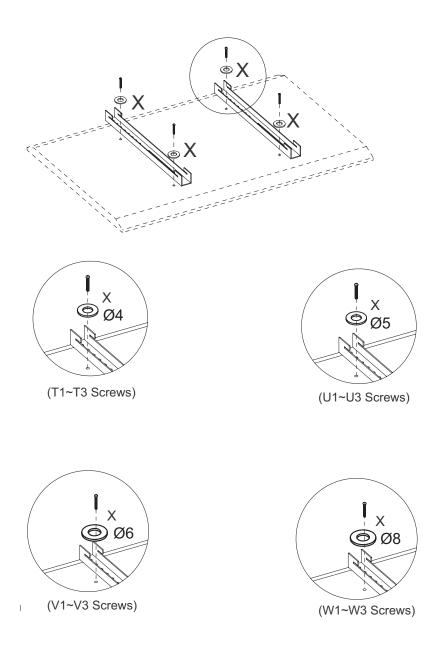
7-Insert Machine Screws through Dual-Hole Washers (X) (see Mounting Hardware list), then into appropriate hole locate on left and right mounting brackets(H), and then into TV.
